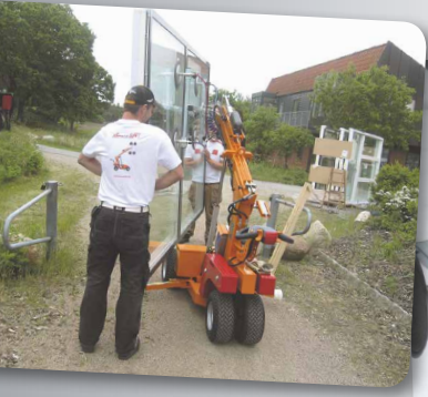
The SL 380 Outdoor is fitted for window and glass installation as standard, but can be supplied with a special device for lifting e.g. heavy fire doors and gates.
